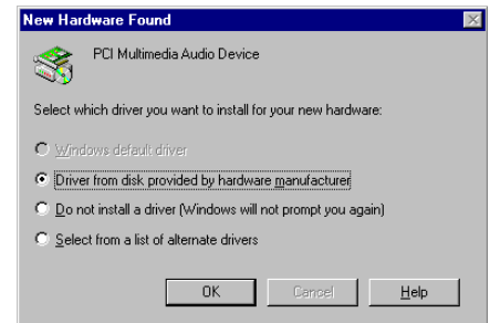
Figure 2-2: Driver installation dialog box where the Windows default driver option is not available.
