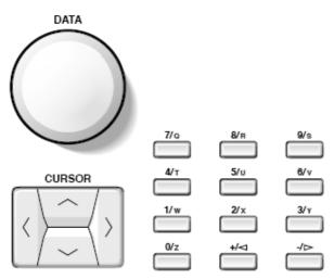
The cursor moves around the various screen options, whilst the data wheel changes the value. The keypad allows for the direct input of values.
