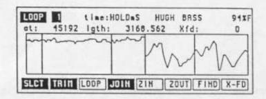
LOOP: First select the loop number that you want to set (top left). Unless you set the loop time to HOLD, loops will be repeated in numerical order. It is not possible to set a loop inside a loop.
