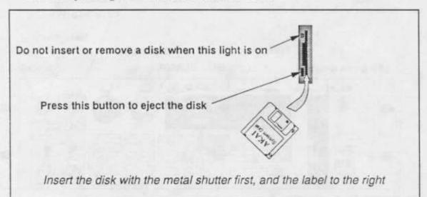
Insert the disk until it clicks into place. To eject a disk, press the black rectangular button at the bottom of the disk drive. When the S1100 is reading or writing a disk ("accessing"), an LED on the disk drive will show this. NEVER try to insert or remove a disk while this light is on! You may damage the drive and/or the data on the disk if you do this.
